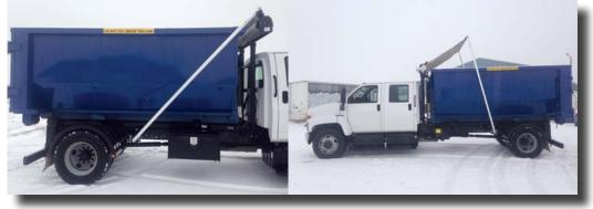
operated. Some examples of semi-automatic tarp system would be an arm-less tarping system similar to a Hy-Tower system or hand crank system that is mounted directly on the container or some type of gantry on the roll-off truck frame.
