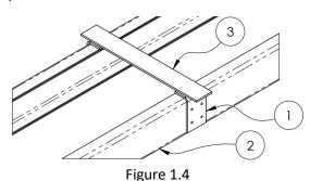
Mark and drill 4 holes per side, taking care not to drill through existing equipment such as wires, hoses, or brackets. Center top plate (3) on mounting brackets side to side and fore/aft. Weld in place. (Figure 1.5).
