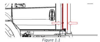
Position supplied mounting brackets (1) on frame (2). Align parts for squarness and ensure clearance between truck cab and all other components (Figure 1.2). Top of bracket should be flush with top of frame rail.
